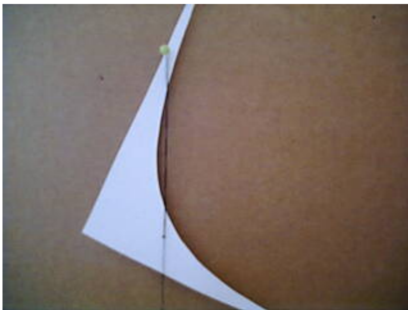
Figure 21: Estimating the centroid using a plumb line.
